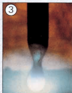
High speed photographs of globule-shedding (SG 2 steel wire, diam. 1,2 mm)
