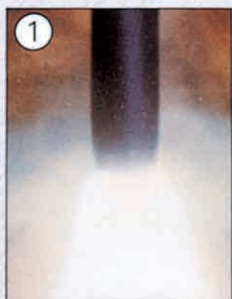
High speed photographs of globule-shedding (SG 2 steel wire, diam. 1,2 mm)
