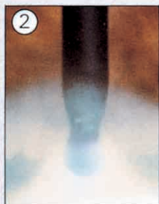
High speed photographs of globule-shedding (SG 2 steel wire, diam. 1,2 mm)
