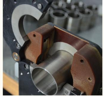
(closed chamber) which results in welds with very limited colouration. They are recommended for welding stainless steel tubes of wall thickness <3 mm in simple fusion without added wire.
